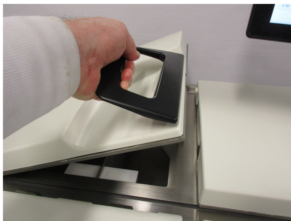
Figure 2-13: Opening a wax bath lid
